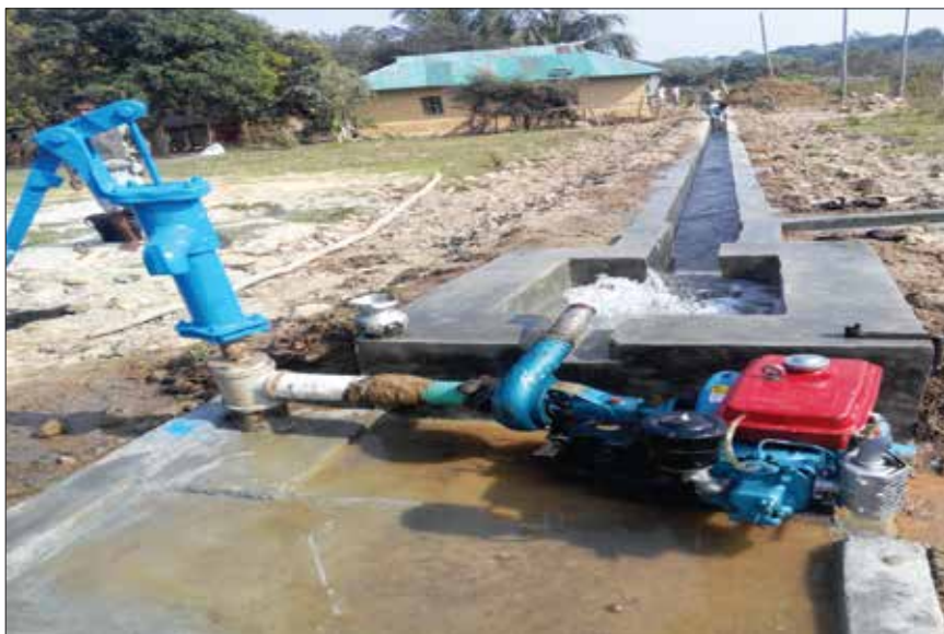
Figure 14 A power pump and a canal at Dayal Kumar para in Manikchari Upazila
